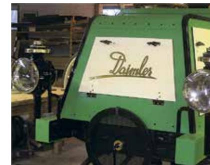
23. Front end of the truck with the brass Daimler nameplate (cut with a laser) and two single-candle headlights installed. Note replica engine crank and flywheel.
