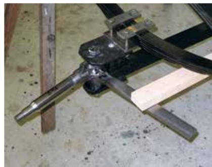
10. In this view, potential front axle and steering problems are shown in the process of being ironed out. The tie rod measurements are also taken at this time.
