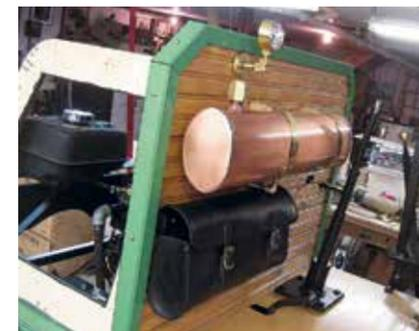
22. Closeup of the truck's finished dashboard with the leather glove compartment, copper gas tank and bronze oil-pressure gauge installed.
