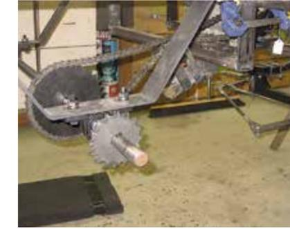
15. Drive chains and chain sprockets had to be tested in conjunction with the engine to ensure the arrangement would transmit the proper speed to wheels.
