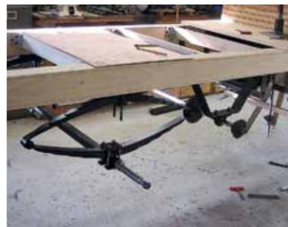
11. Next, the rear leaf springs (buggy springs made by Amish craftsmen) and axle are bolted in place beneath the truck's body.
