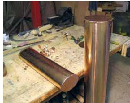
5. The next step is to form the copper gas tank and then test fit the crimped ends on both tanks prior to soldering them both tight.
