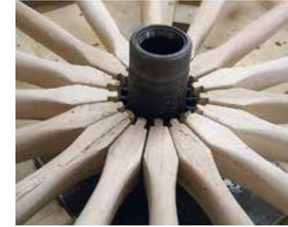
14. All of the wheel spokes dovetailed and inserted into the Amish-made metal axle hub in preparation for being bolted through the metal wheel hub.
