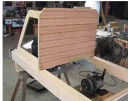
7. The finished dashboard is installed on the passenger side of the plywood bulkhead. Note initial test placement of the transmission and clutch.
