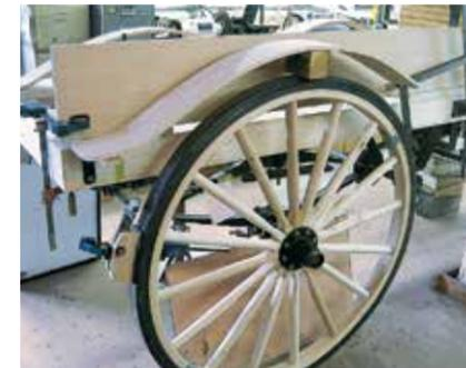
19. Test fitting the steam-bent ash-wood fenders to the Daimler truck's body.
