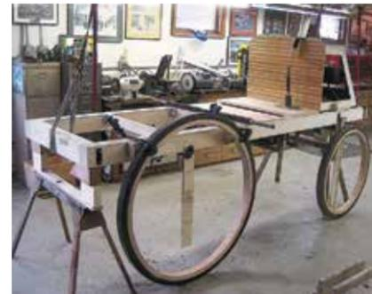
9. Establishing the correct location for the wheels. Proper steering angles and spring size must be determined, along with resolving a host of other mechanical issues.
