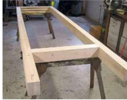
1. The 1898 Daimler truck's basic frame is built from two 2x6 beams of laminated poplar, the same wood used in the construction of early Concord stagecoaches.
