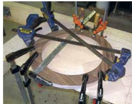
8. The steering wheel is initially cut out roughly with a bandsaw from walnut and then assembled and glued up in two laminated layers.
