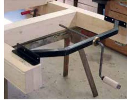
3. Fitting the fabricated metal brace to stiffen the front end, act as an engine mount and locate the engine crank.
