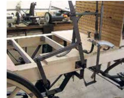
17. Positioning, attaching and connecting up the 1898 replica's two small stagecoach-style shoe brakes.
