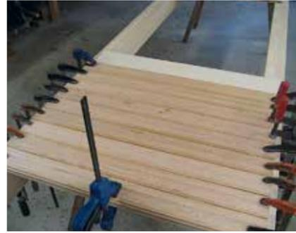
2. Using the poplar frame as a handy flat and true surface, the next step is to glue together the truck's dashboard out of traditional tongue-and-groove red oak bead board.
