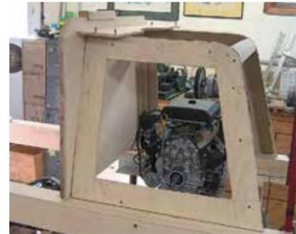
6. Test fitting the modern engine after framing out the truck's front end in plywood. Sheet-metal cladding will be installed on top of the plywood frame.
