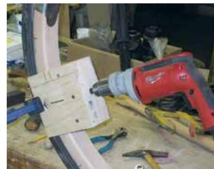
12. Drilling the Amish-made metal-edged wooden wheel rims to accept the wooden spokes, using basic geometry and a shop-made drilling jig.
