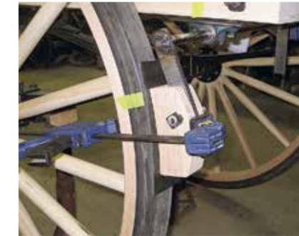
18. Historic engineering on the fly: sorting out the correct positioning of the rear shoe brakes.
