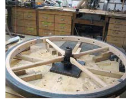
13. Installing the first wooden spokes into the wooden wheel rims and axle hubs. Ash wood was a traditional material choice from which to make wagon-wheel spokes.
